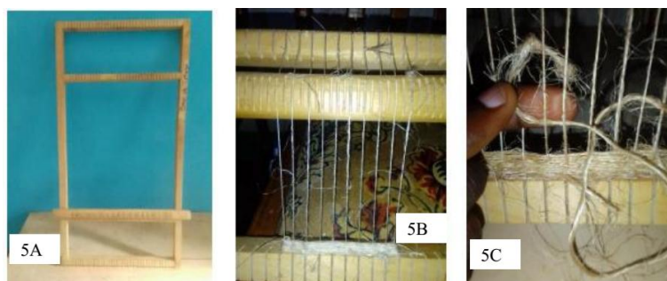
Figure 5. Stages in the production of woven membranes from banana pseudo-stem fibres (loom (5A), warp, weft yarn (5B) and weaving (5C).
