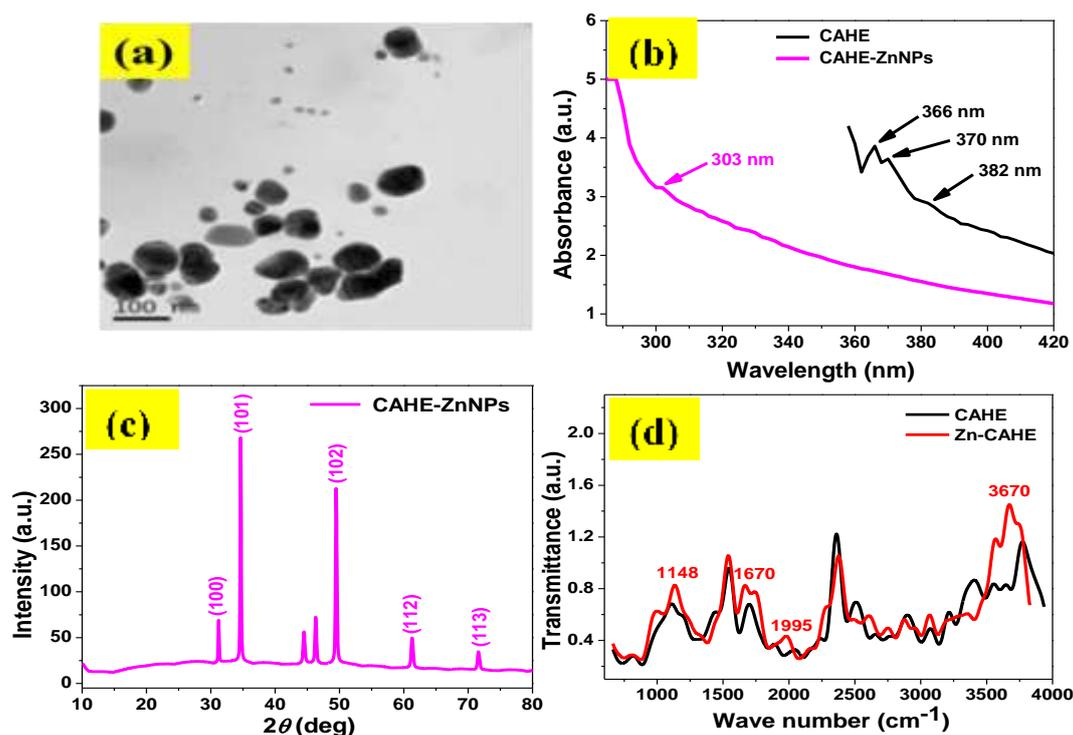
**Figure 3.** (a) TEM image of CAHE; (b) UV-Vis spectra of CAHE (black) and CAHE-ZnNPs (purple); XRD diffraction pattern of CAHE-ZnNPs; and (d) FTIR spectrum of CAHE (black) and CAHE-ZnNPs (red).
